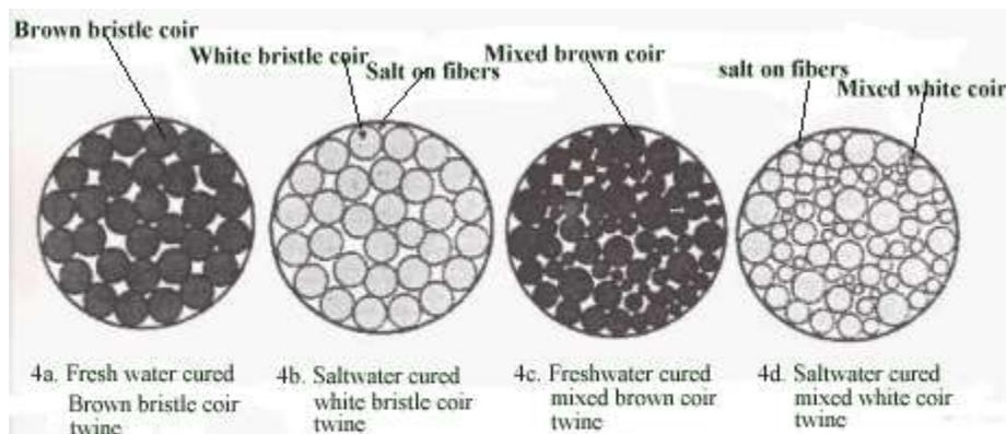
**Figure 4. Enlarged cross section of currently available different types of coir twines**
